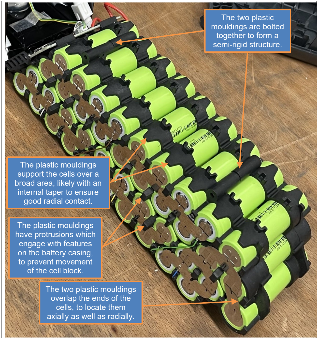
Figure 57: The Cell Support Structure in Product #6
