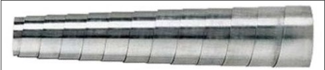
Figure 17: Exaggerated Example of a Telescoped Spiral (from Hennig (UK) Ltd., 2015)
