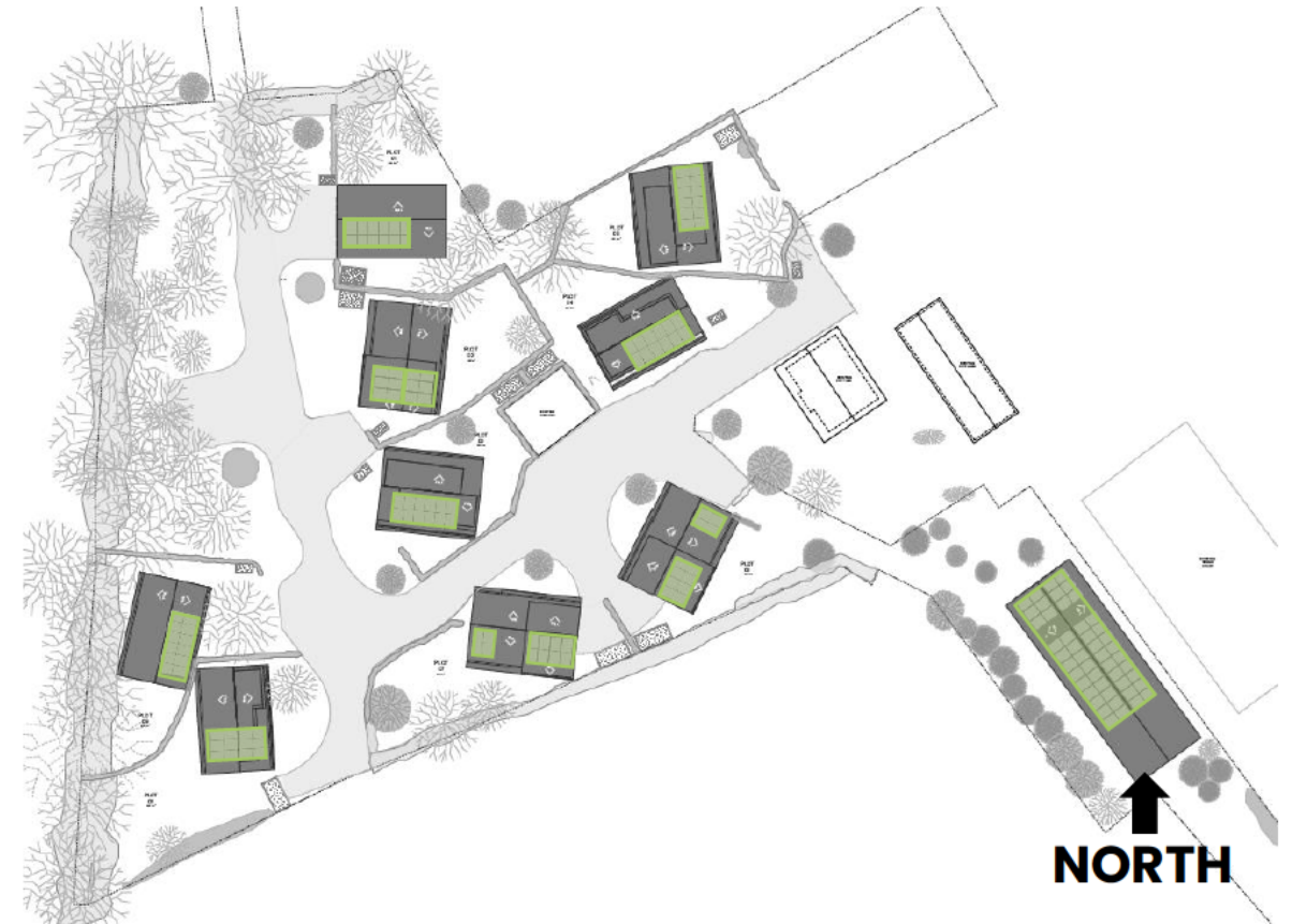
Figure 7: Space allocated for Solar PV (green).
