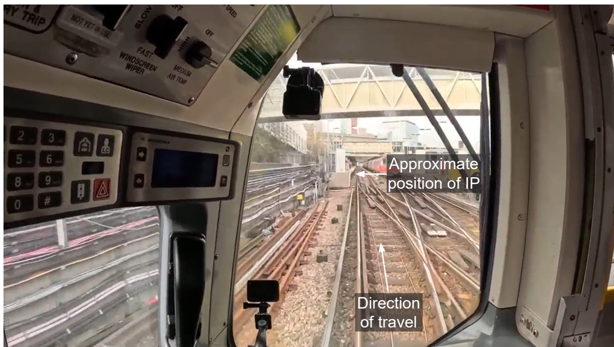
Figure 9: The moment that the reconstruction TO stated they would have recognised the obstruction as a safety risk and applied the emergency brake, approximately 40 metres from the object.
