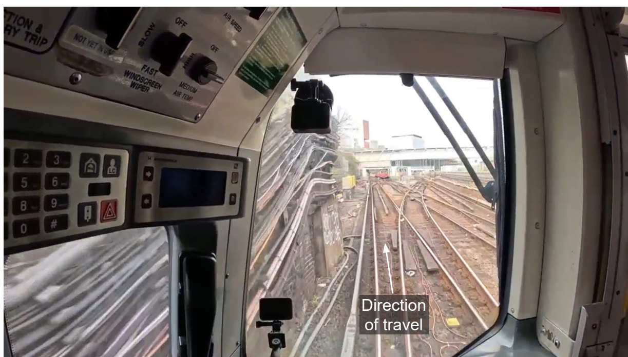
Figure 8: The moment that the reconstruction TO was able to recognise the reference object on the track, approximately 112 metres from the object.
