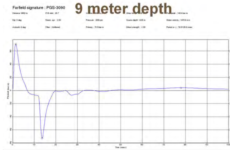
Figure 5: Farfield signature: PGS-3090; 9 m depth: Airgun signature in bar metres (bar m) (supplied by W Pramik, Geokinetics).
