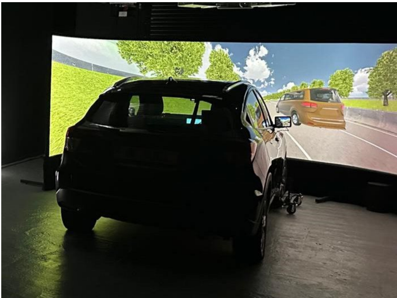
View of the UCL simulator's exterior showing the rear of the vehicle and the simulated scene of the road ahead on a 180-degree curved screen.
