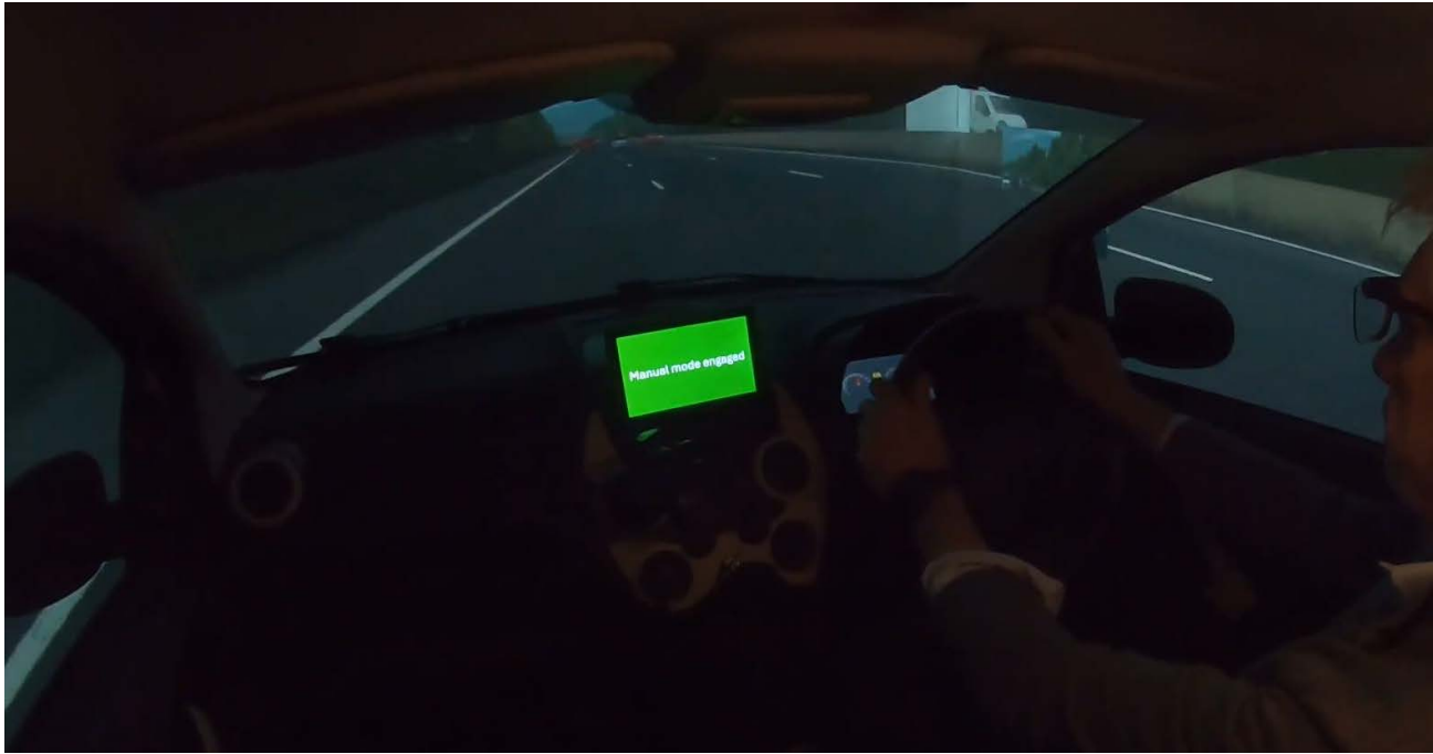
Participant with both hands on the steering wheel and the display screen showing “Manual mode engaged” with the simulated screen showing the road ahead.
