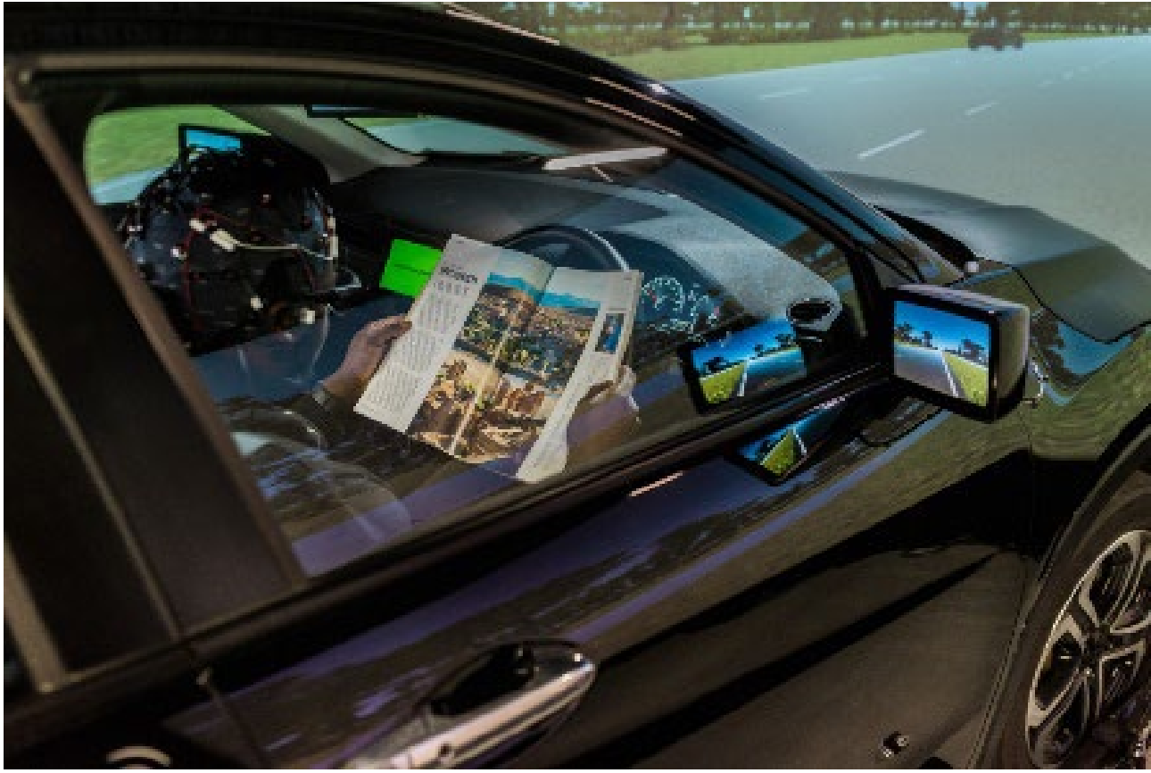
A participant in the UCL simulator, reading a magazine while completing one of the NDRA activities. The participant is wearing an EEG cap and eye-tracking glasses.
