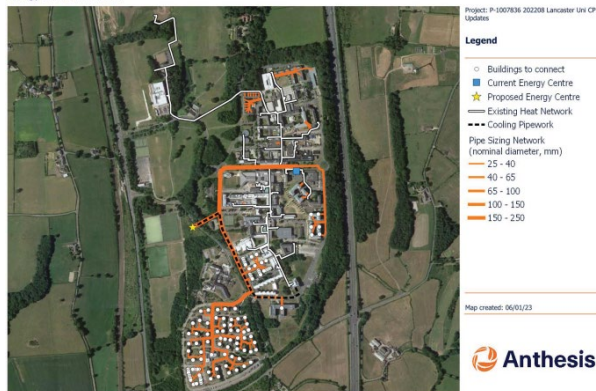
Pipe Sizing Energy Centre Location E
