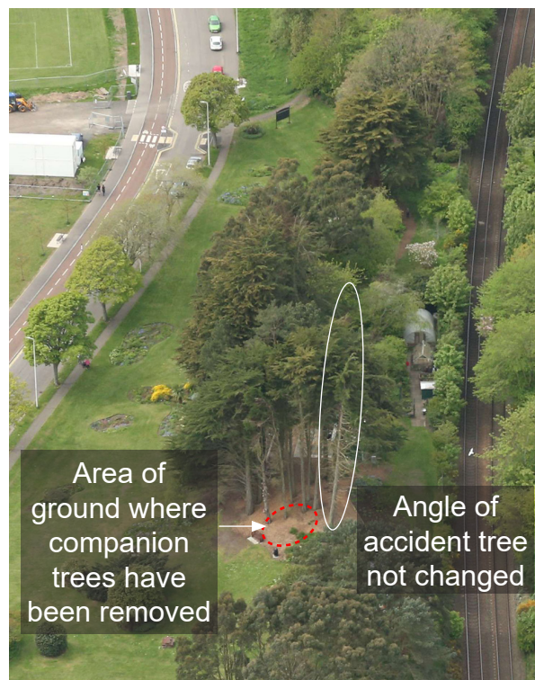
Figure 16: Network Rail aerial image showing the trees in May 2023 (courtesy of Network Rail with RAIB annotations).
