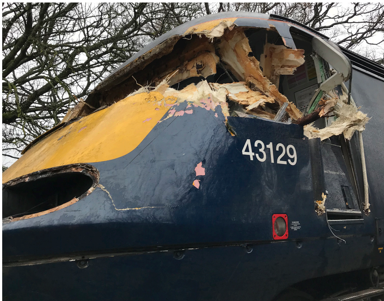
Figure 6: Damage sustained to left-hand side of driving cab.
