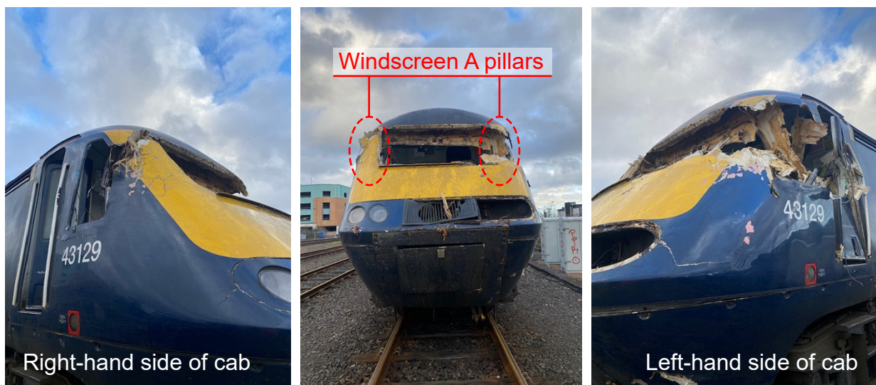
Figure 20: External damage sustained to leading power car of 1A37.
