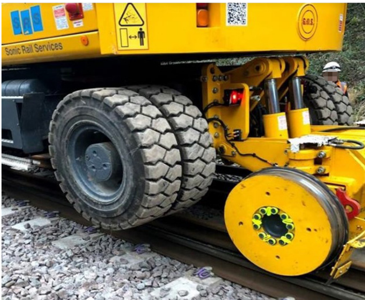
Figure 11: An RRV of the same type showing the overhang of the rubber tyre in relation to the rail (courtesy of Sonic Rail Services).
