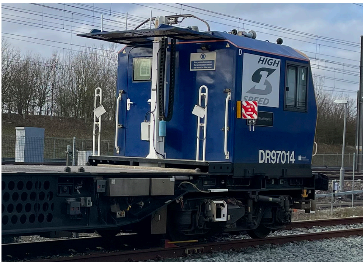
Figure 9: The rear of an HS1 MPV cab. On the night of the accident a container was mounted on the rear deck.
