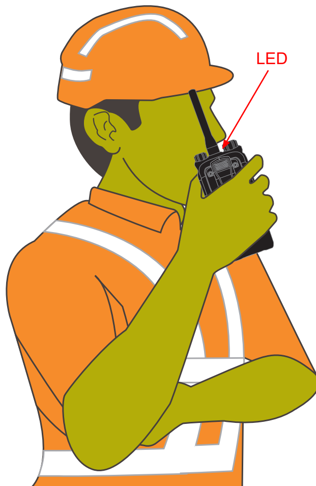
Figure 11: Radio held in a talking position, making the LED difficult to see.
