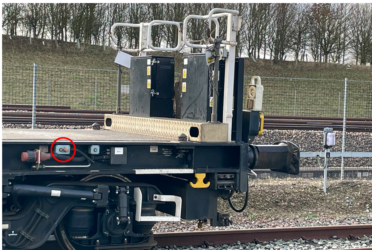
Figure 12: The emergency stop buttons fitted to the sides of HS1 MPVs.
