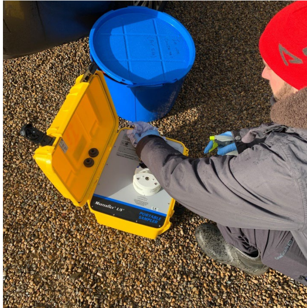
Figure 15. Peristaltic pump being cleaned with 10% bleach solution
