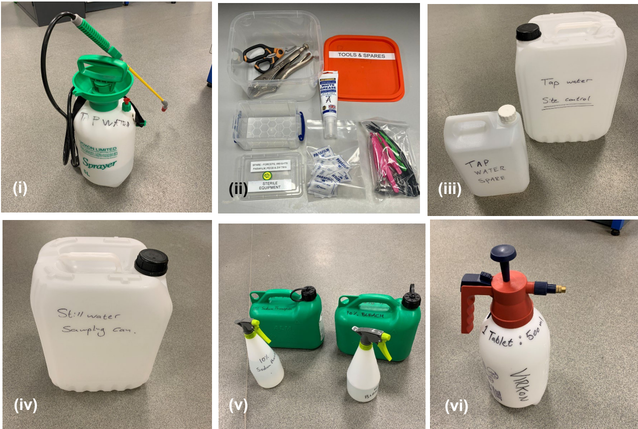
(i) 5L pump sprayer holding tap water, (ii) Tools and spares containers. Sealed container with spare parafilm and forceps. Grease for pump and shears and locking pliers. (iii) 20L Site control jerry can and spare 5L water jerry can, (iv) still water sampling can for collecting and homogenising sample, (v) 5L jerry cans and hand sprayers containing 10% solutions of bleach and sodium thiosulphate, (vi) virkon spray bottle for disinfection between sites.
