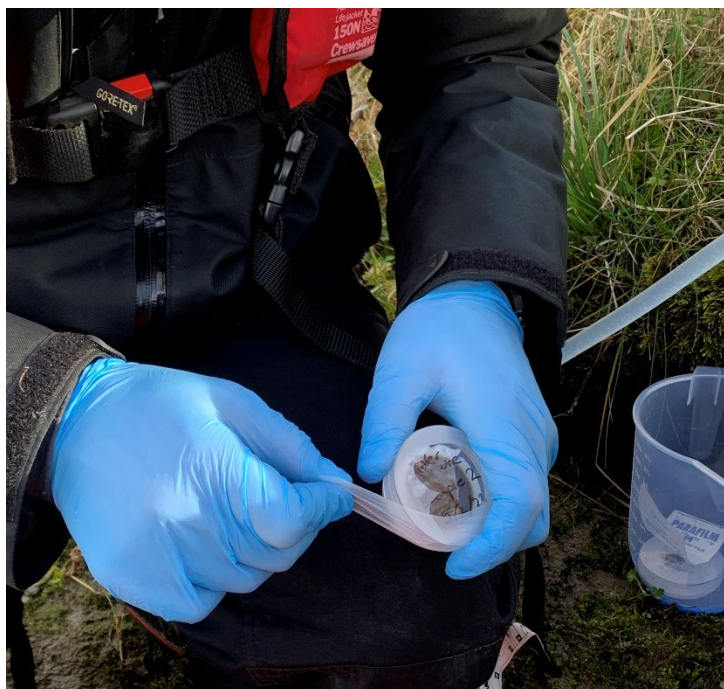
Figure 14. Applying Parafilm M to Petri dish [Step 22].
