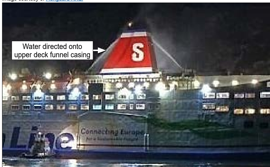
Figure 3: Boundary cooling of Stena Europe's funnel casing
