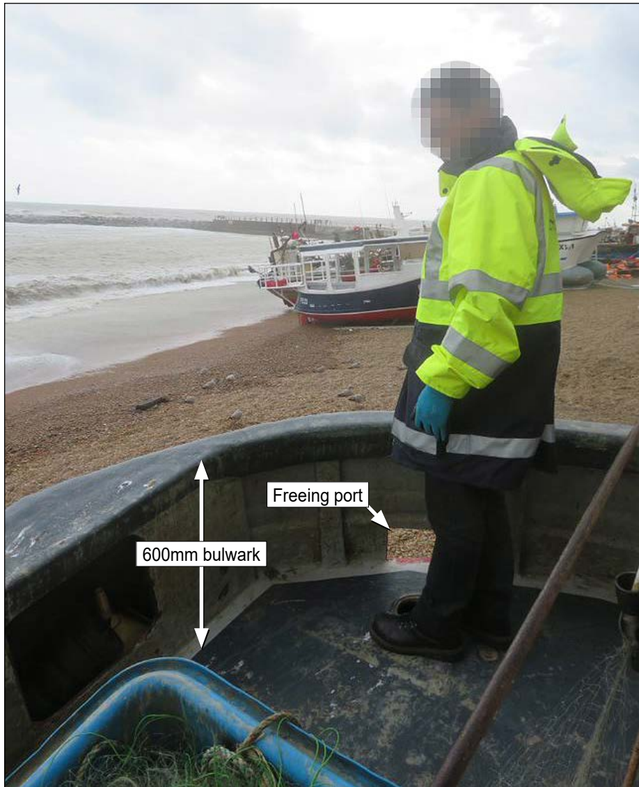
Figure 3: View of aft deck bulwark with a person who is 172cm tall standing adjacent
