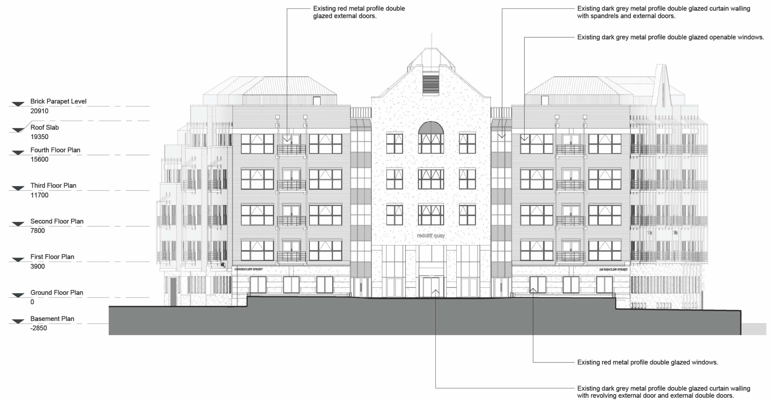
6 Existing Building - Elevation 6 - Planning 1 : 200
