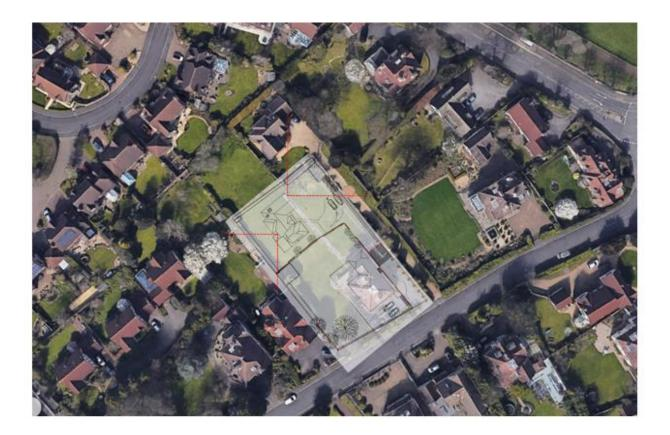
As is illustrated, the proposal would not breach the 45-degree angle to the mid-point of habitable rooms at neighbouring number 6.
