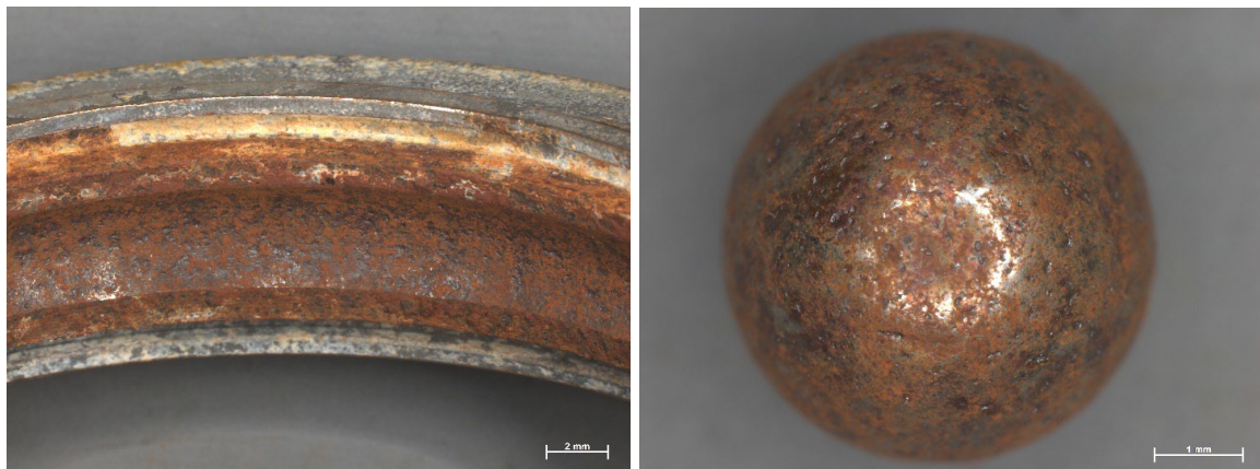
Figure 7 Bearing No 2 corrosion and pitting (outer race shown, inner similar)
