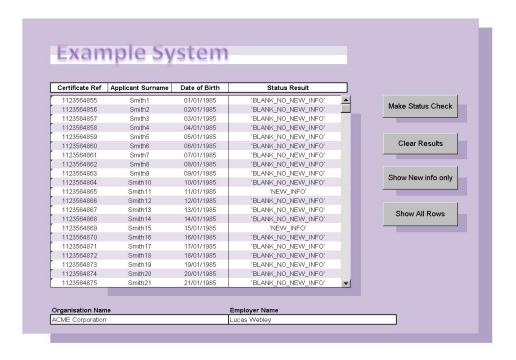
The input data used to construct the URL (mandatory information relating to the individual's DBS certificate) is captured in the first three columns of the table.
