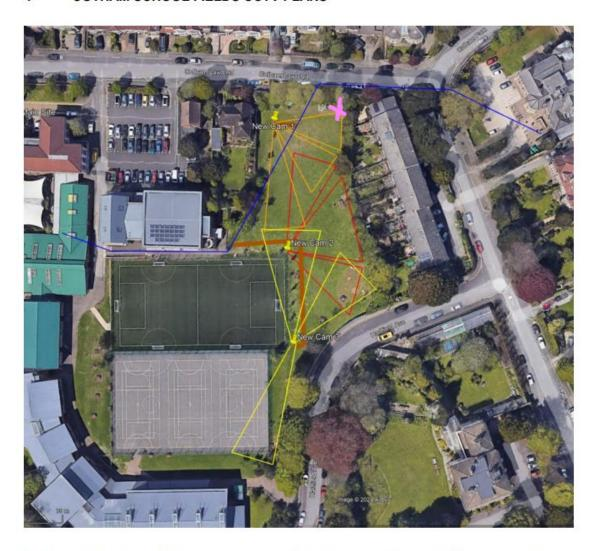
New Cam 1, New Cam 2 & New Cam 3 locations have been decided so as to take into consideration proximity to trees / roots, domestic residences, bat surveys etc. (Existing duct route indicated in Blue, proposed new cable routes indicated in Brown).
