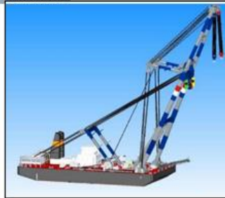
Sheerleg with gangway and extra accommodation installed
