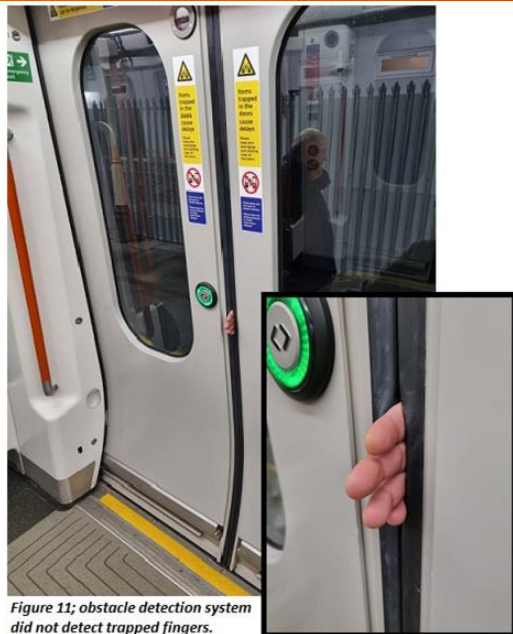
Figure 10; fingers trapped in 710 doors, in fully closed position.
