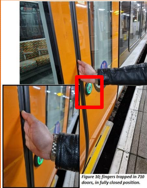
Figure 11; obstacle detection system did not detect trapped fingers.
