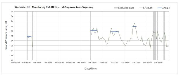
Note: Missing data throughout the week was due to a loss of power to the monitoring station caused by vegetation overgrowth preventing sufficient light reach the solar panel.
