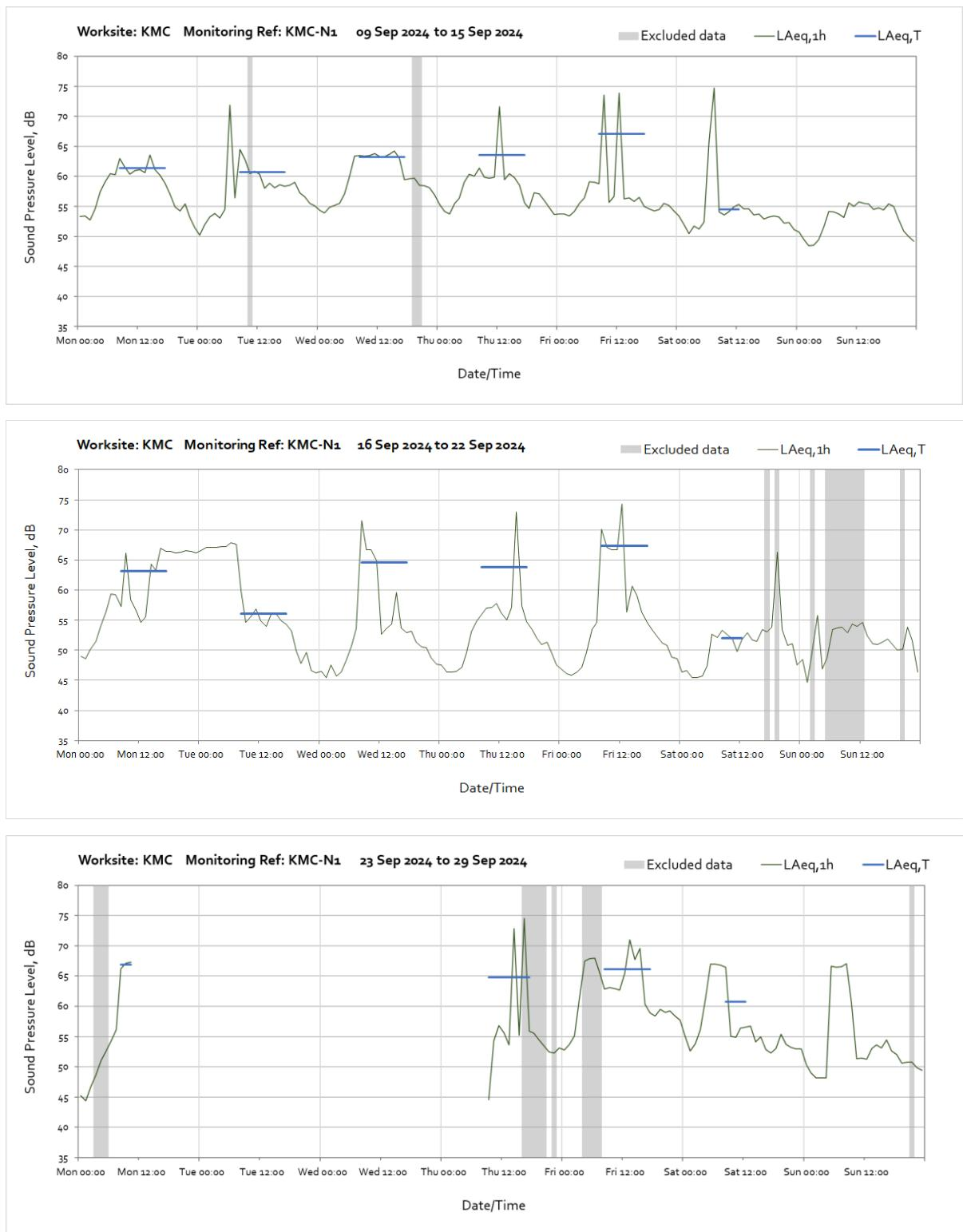
Note: Missing data between 11:00 on Monday 23<sup>rd</sup> and 09:00 on Thursday 26<sup>th</sup> September was due to a remote reset error causing the monitor to remain offline until manually reset.
