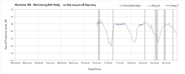
Note: Missing data from the start of the month until 11:00 on Thursday 05<sup>th</sup> of September was due to a loss of power to the monitoring station caused by poor weather conditions preventing sufficient light reach the solar panel.
