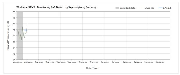
Note: Missing data from the 12:00 on Monday 23<sup>rd</sup> of September until the end of the month was due to loss of power at the monitoring station.
