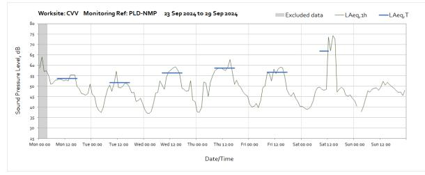
Note: Missing data between 01:00 and 03:00 on Sunday 29<sup>th</sup> of September was due to a communication error between the monitoring station and the server.
