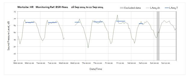
Note: Missing data between 02:00 and 11:00 on Wednesday 18<sup>th</sup> of September was due to loss of power at the monitoring station.
