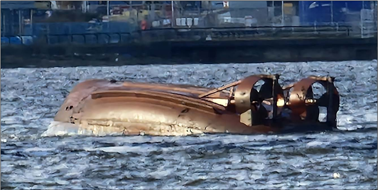
Figure 6: Biter capsized with its rudders set at approximately 30° to starboard
