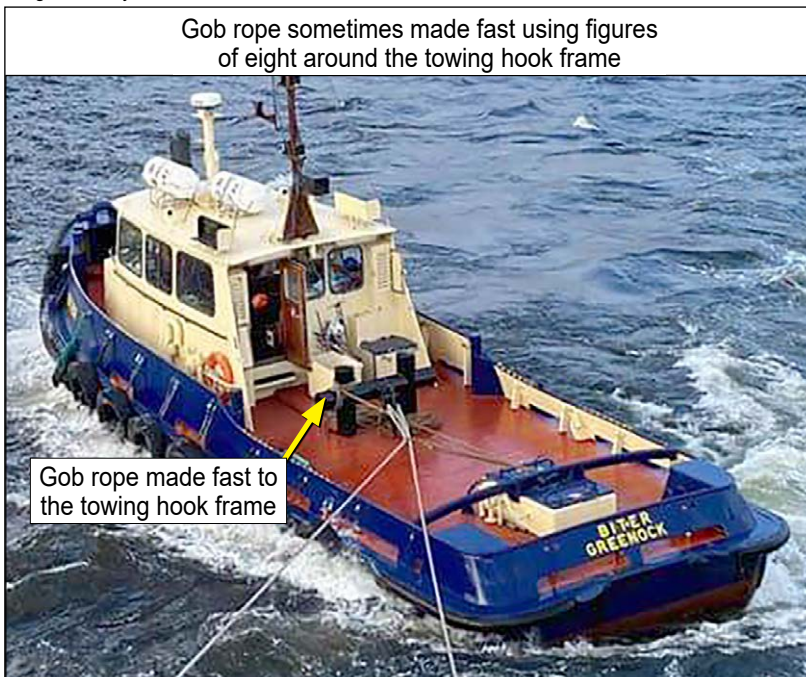
Figure 9: Biter's towing arrangements
