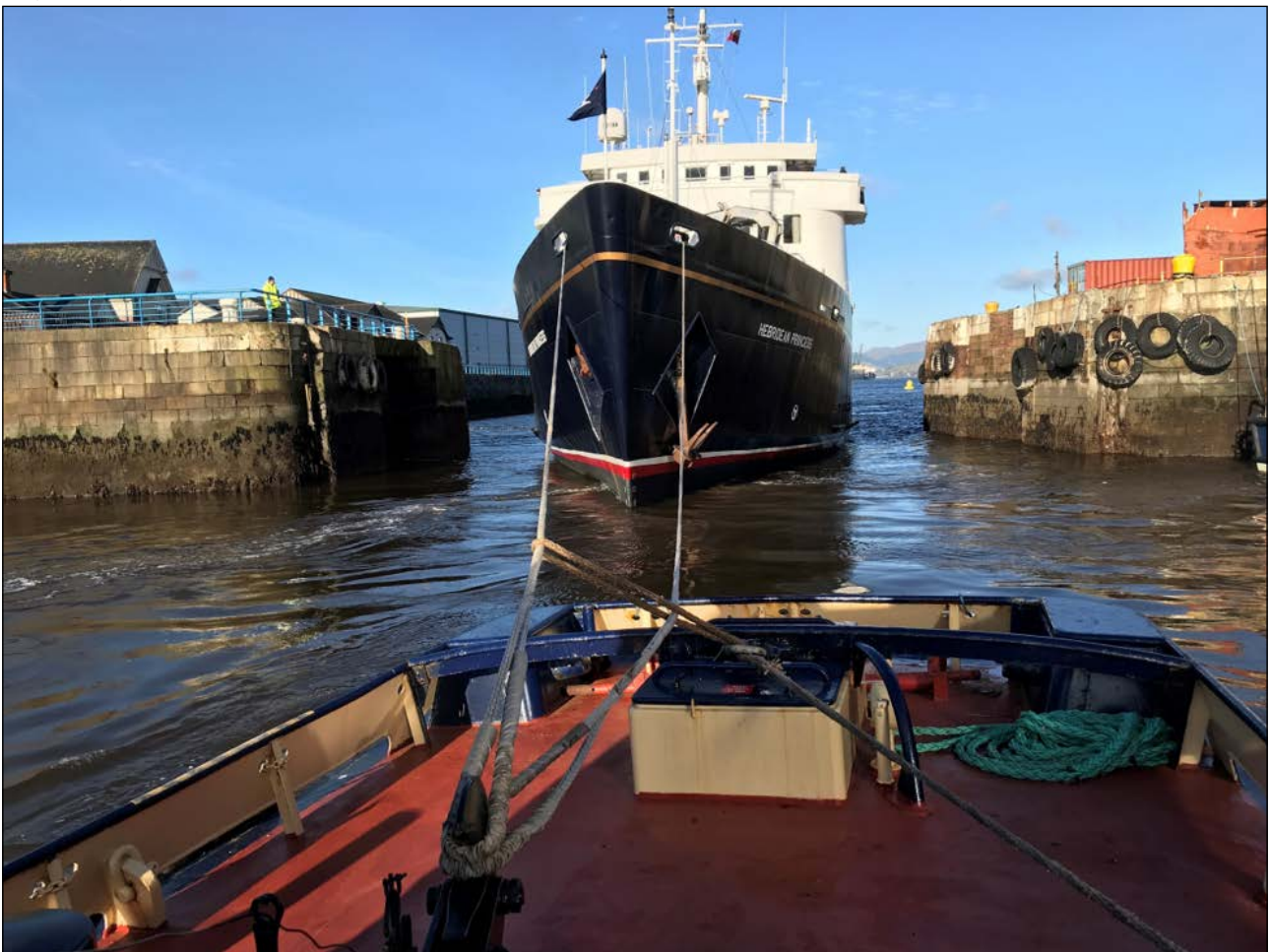
Figure 13: Biter 's gob rope while assisting Hebridean Princess to leave James Watt Dock on the morning of 24 February 2023
