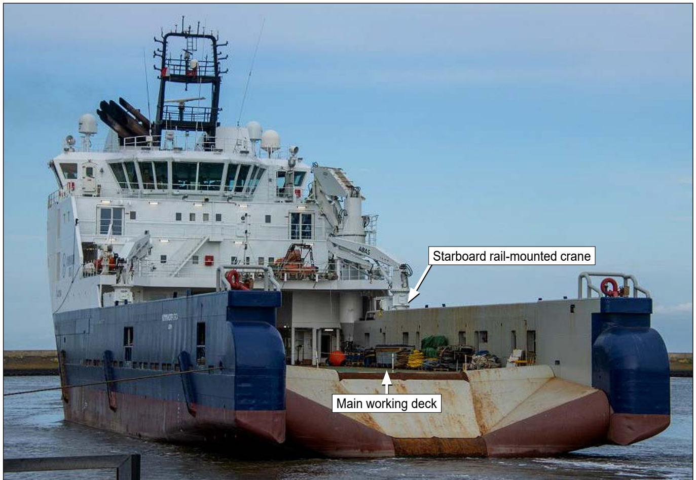
Figure 1: Kommandor Orca 's deck arrangement
