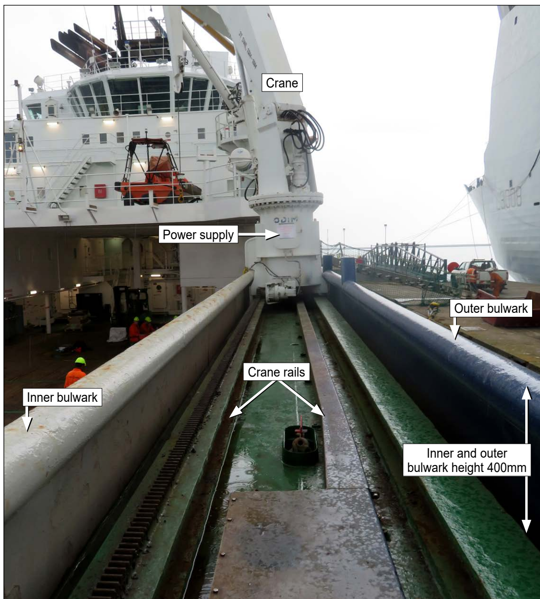
Figure 2: Starboard rail-mounted crane
