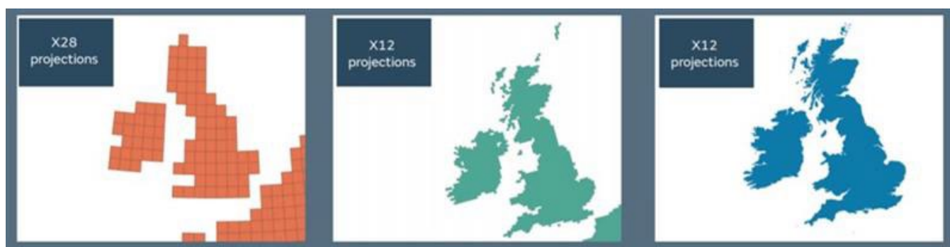
Figure 2. Maps showing the resolution of the global (orange), regional (green) and convection-permitting (“CPM”) climate models used to produce the UKCP18 climate projections. The inset boxes indicate the number of ensemble members. The global projections include 15 versions of the Hadley Centre’s model HadGEM3-GC3.05 and results produced by 13 models from other climate centres. This image © Crown Copyright 2018.
