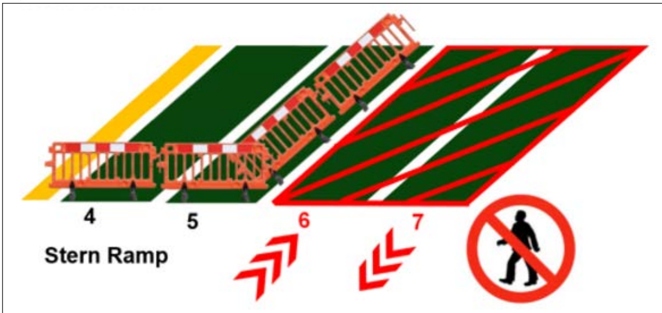
Figure 18: Extract from Seatruck's Deck and Safety Procedures Guide, showing a lower hold designated walkway and lane makings
