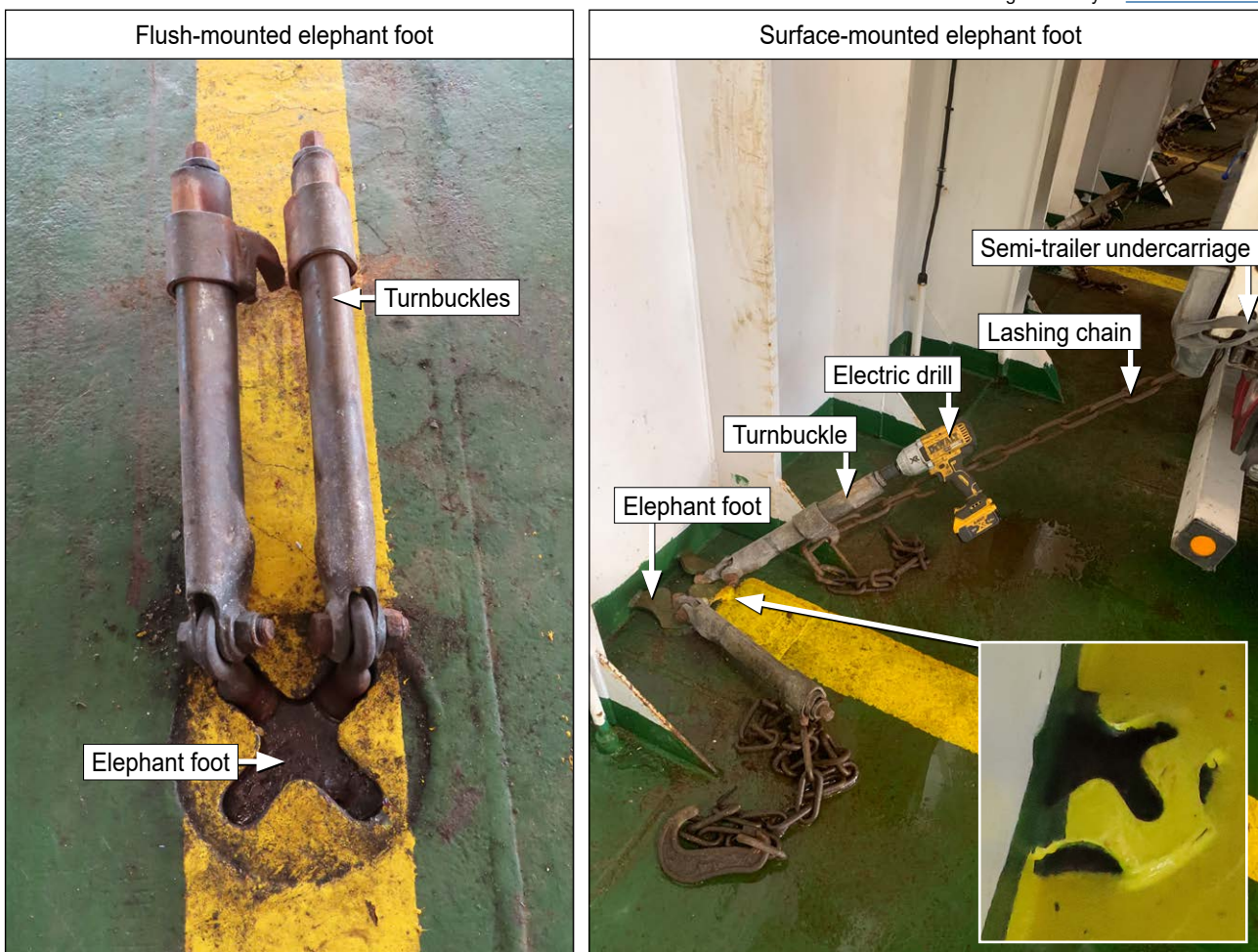
Figure 8: The elephant’s feet securing arrangement
