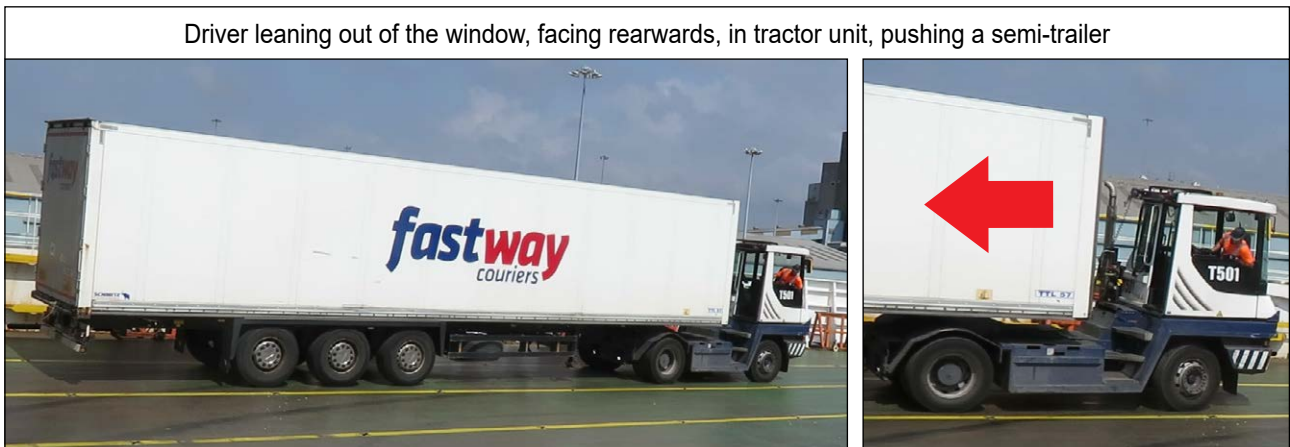
Figure 14: Reconstruction of the tractor unit driver positions when pulling and pushing a semi-trailer
