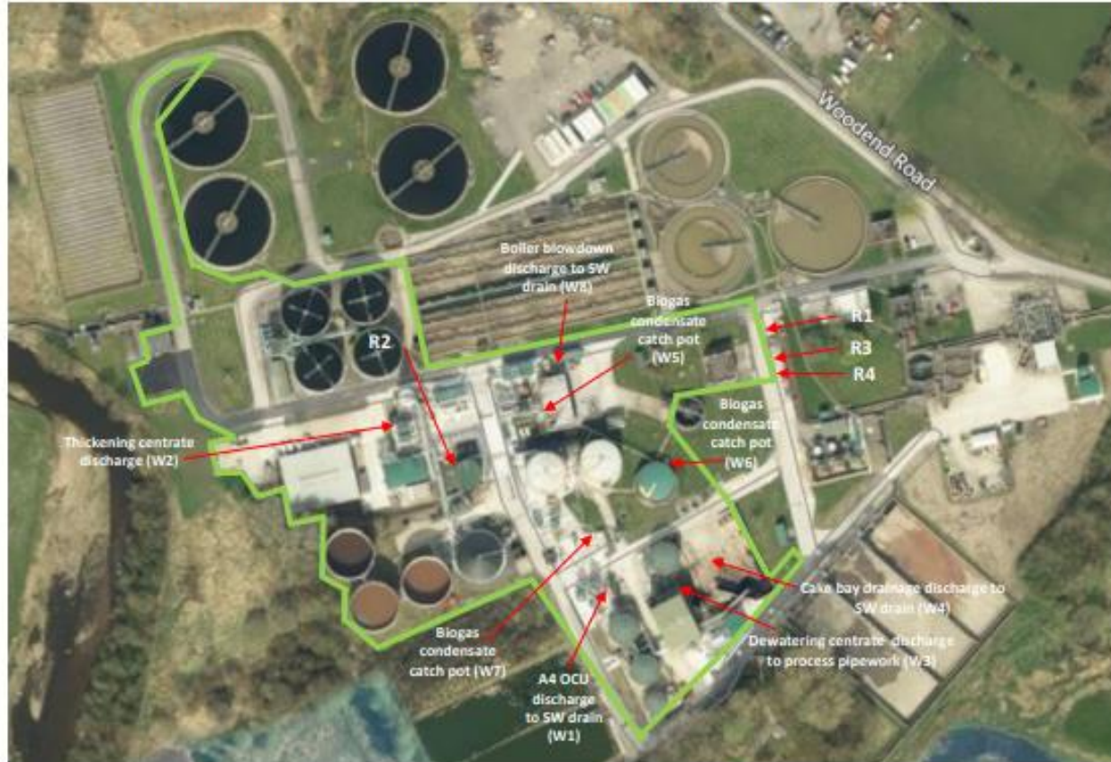
Appendix E Figure 3 - Burnley WwTW Sludge Treatment Facility Wastewater Emission Points – Returns to WwTW (Updated September 2024)
