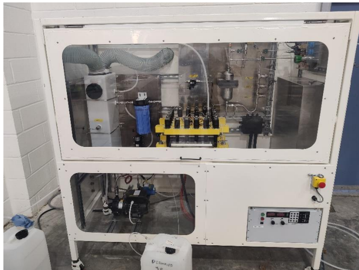
Figure 3. High pressure operational test bench
