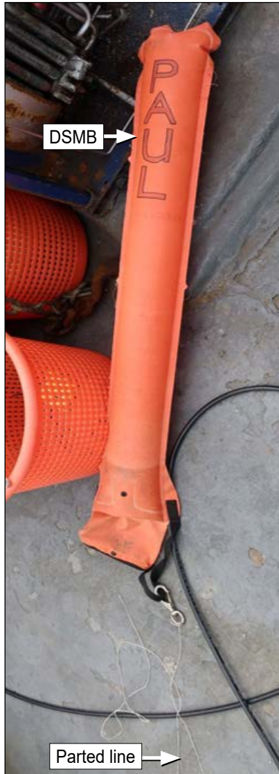
Figure 2: Diver 1's marked DSMB with its parted line and hand reel of a similar type to that used by diver 1
