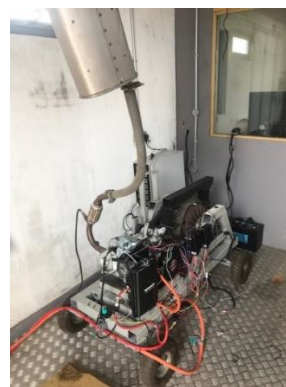
Figure 2: 6HGE test cell and dynamometer
