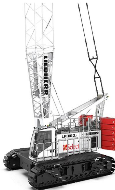
Figure 1: Battery electric crane the fuel cell gen-set is designed to charge 7
