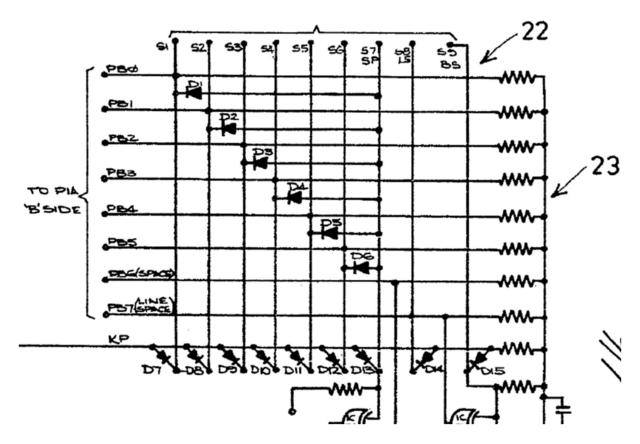
55. From Fig. 7 and the associated description (page 3 line 11 to line 76) depressing a first key S1-9 will activate an output PB0-7 to the PIA of Fig. 6 (see discussion relating to claim 1 above) and the KP (key pressed) line. The key pressed line feeds a delay circuit (shown in another part Fig. 7 not reproduced) which outputs a strobe signal telling the computer section shown in Fig. 6 to read the lines PB0-7. This is described on page 3 lines 41-49.
