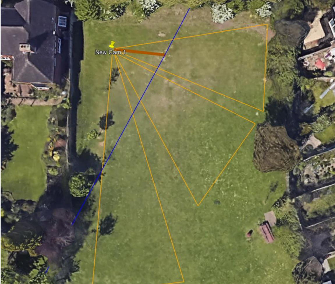
(Existing duct route indicated in Blue, proposed new cable routes indicated in Brown).
