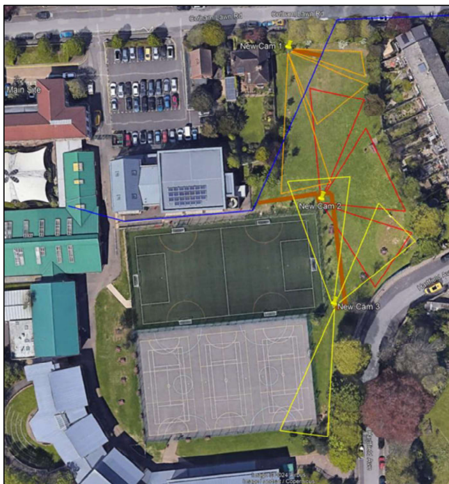
Figure 1: The existing duct route is indicated in blue and the proposed new cable routes are indicated in brown.
