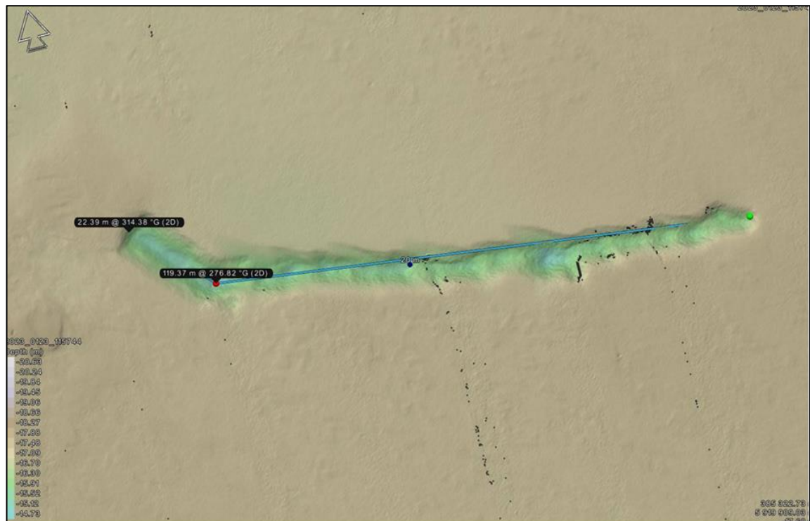
Figure 3-3: Historical rock placement on PL 874/PL 875 within the Guinevere 500m exclusion zone.
