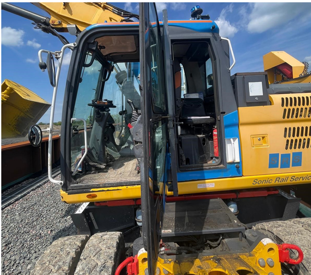
Figure 6: RRV's double cab. The MC sat in the rear part of the cab with limited forward visibility (courtesy of Sonic Rail Services).
