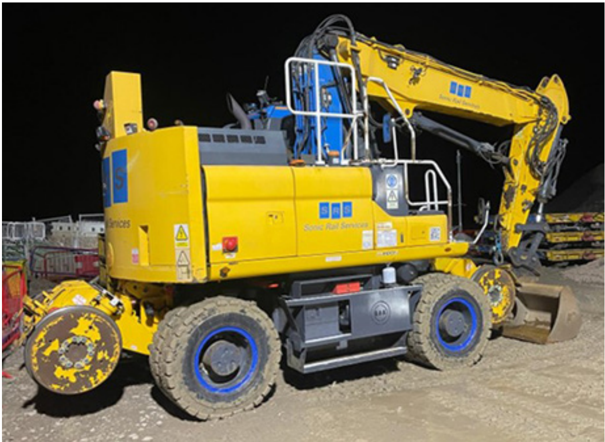
Figure 3: Road-rail vehicle used on 21 to 22 November (courtesy of Sonic Rail Services).
