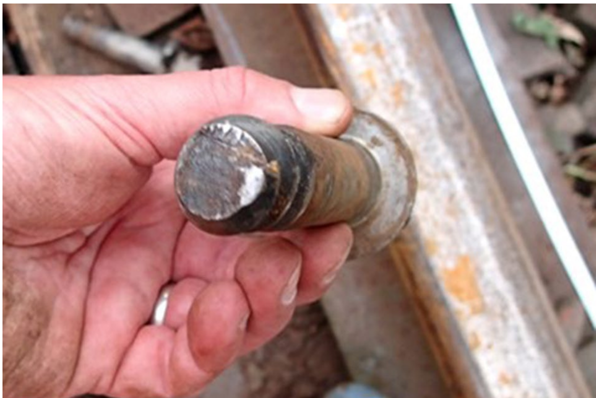
Figure 2: One of the recovered top portions of a screw with signs of historical fracture and subsequent failure by overload (bright area).
