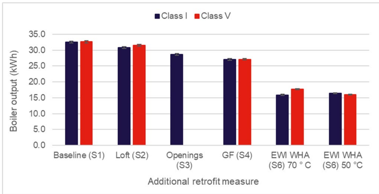
Figure 18: Boiler output at each stage of the piecemeal retrofit using Class I and Class V control and the impact of flow temperature setpoint modification at Stage 6
