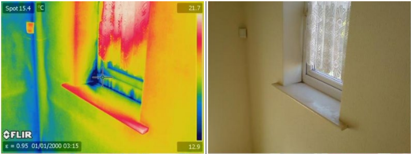
Figure 2-17 Air movement around window casement and seal
