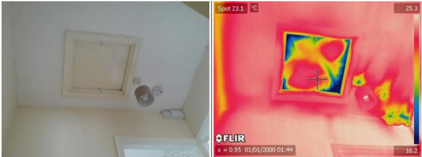
Figure 2-21 Air movement around a loft hatch
