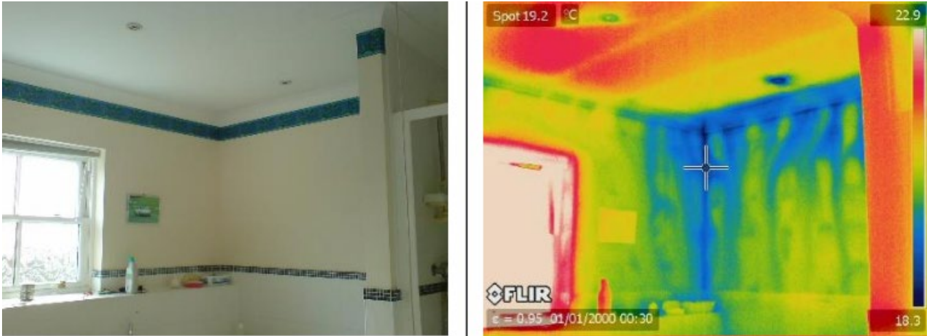
Figure 2-25 Air movement behind plasterboard drylining
