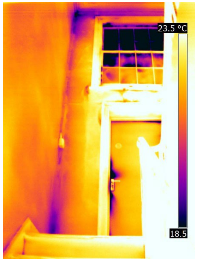
Figure 3-2 Air leakage at the front door of 07LT (moving into the floor void above) and around the first floor door to the rear annex and window above
