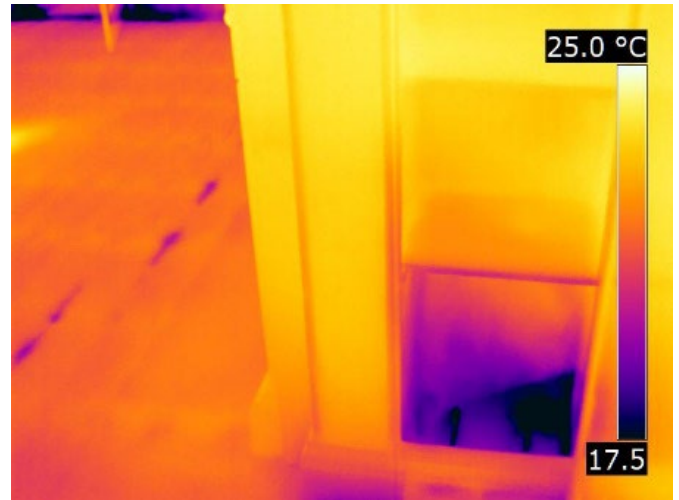
Figure 3-9 Emerging air at the ground floor, coolest at the room perimeter junctions with the external walls and areas of uncarpeted floor
