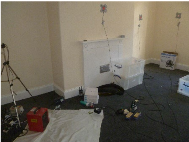
Figure 3-6 Contrasting airtight performance of the fireplaces in Bedroom 1 of 07LT (open) and Bedroom 1 of 09LT (sealed and vented)
