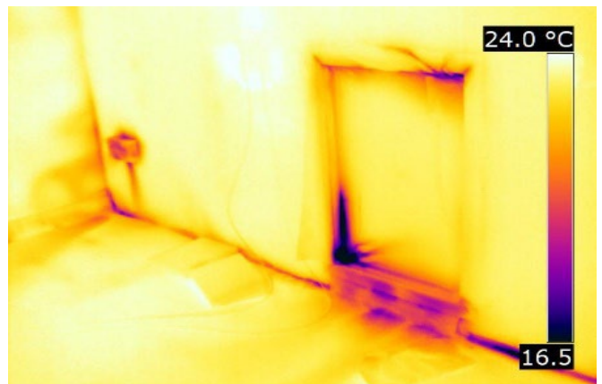
Figure 3-14 The new eaves void access hatches in 07LT, not yet fastened and draught-stripped, at the time of the post room-in-roof retrofit pressure test
