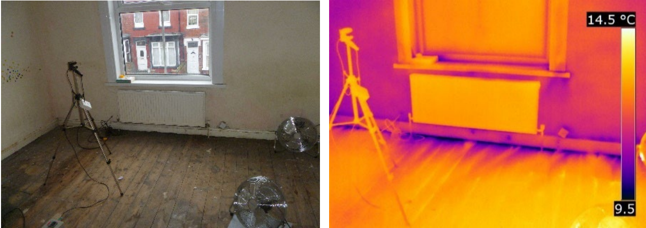
Figure 3-5 Base case infiltration around the perimeter of the intermediate floor during depressurisation
