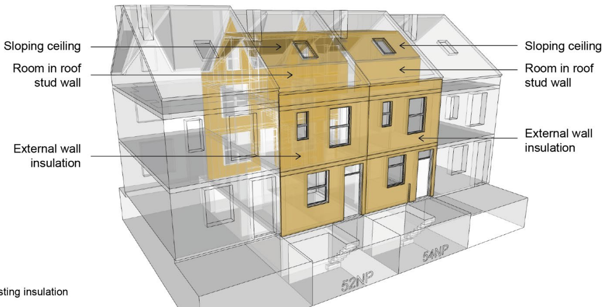
Figure 1-6 Stage 1: Insulation already in the property prior to the retrofits (52NP.B and 54NP.B), front and rear elevations
