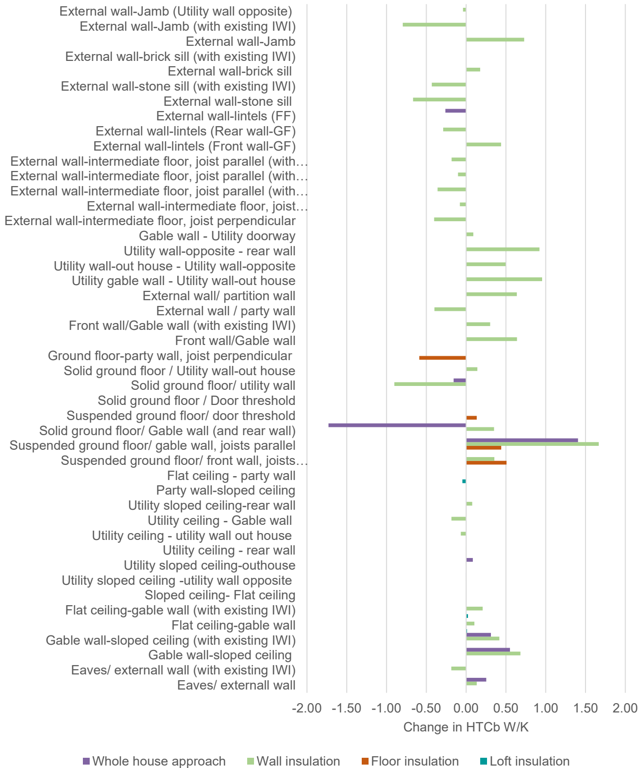
Figure 3-22 change in HTC_b per junction for each retrofit stage (flat ceiling – sloped ceiling junction omitted for clarity)
