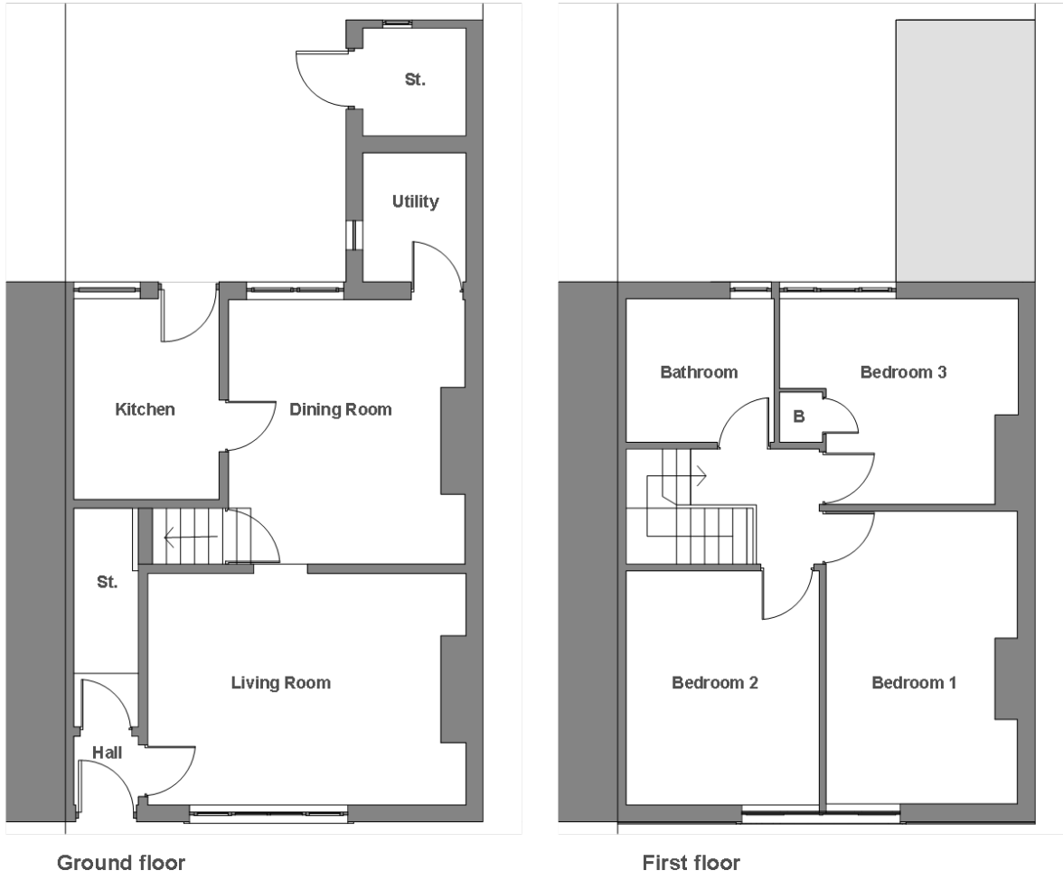
Figure 1-3 House floor plans
