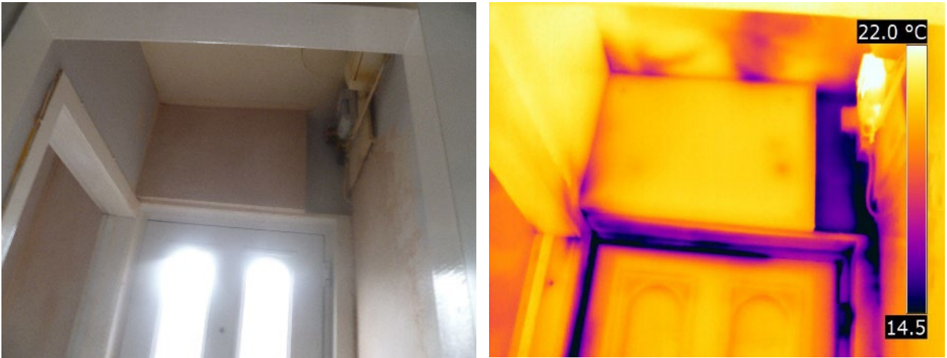
Figure 3-7 Air movement around the front door
