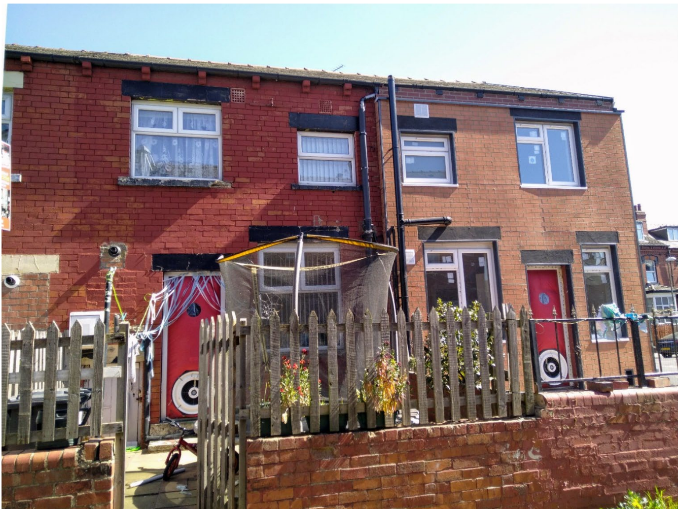
Figure 2-1 Blower doors in adjoining dwellings during co-pressurisation test
