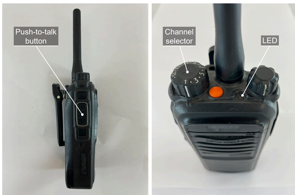
Figure 10: Radio used by the machine controller on the night of the accident, showing LED, channel selector and push-to-talk button.
