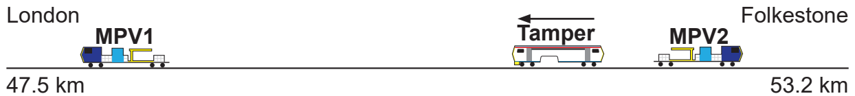
Figure 6: The vehicles' positions as the tamper started work.
