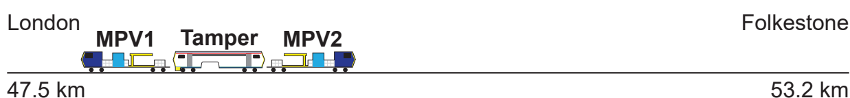
Figure 5: The train at the London end of the work site.
