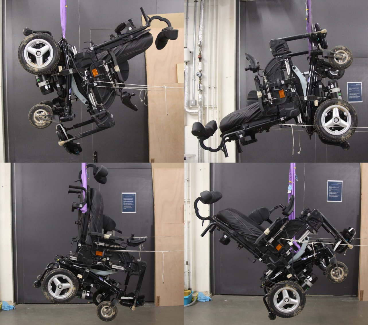
Figure 18 Invacare Bora centre of gravity survey
