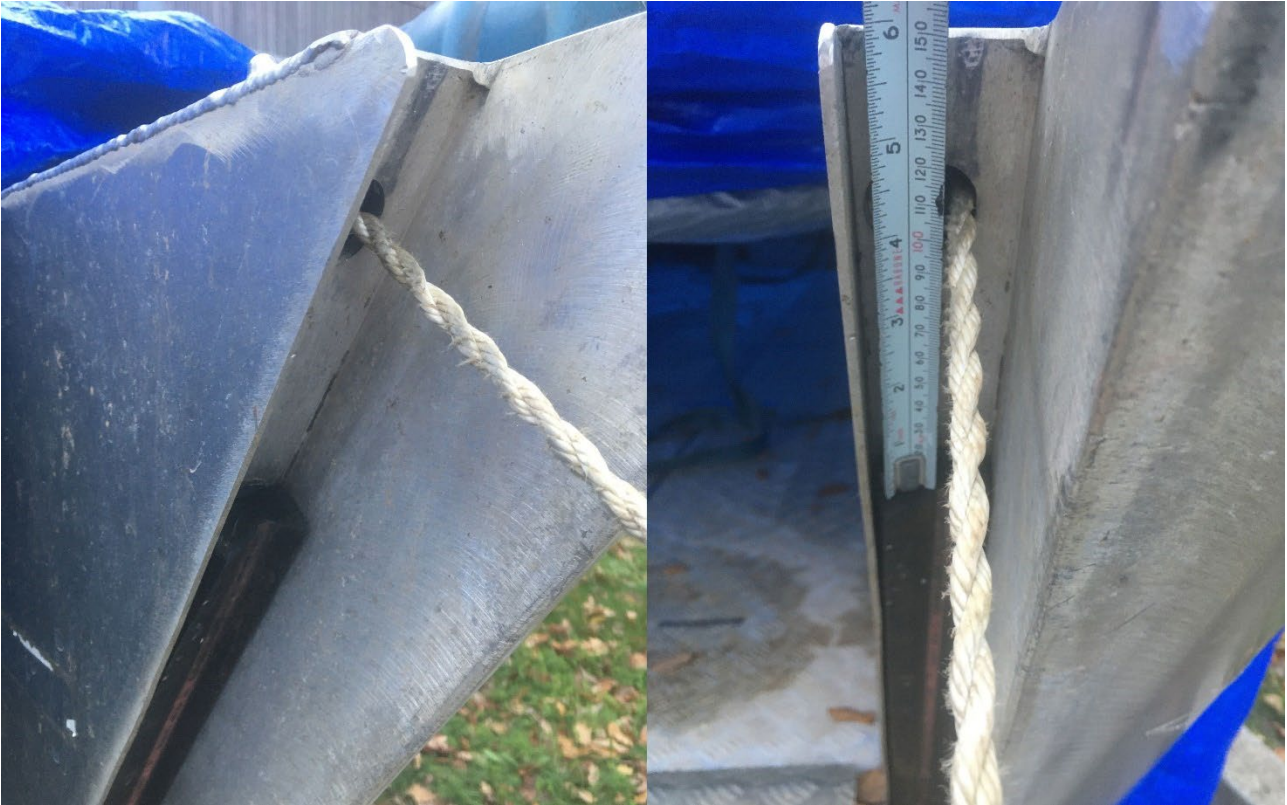
Figure 8 Rubber seal fitted in bow ramp channel, port side
