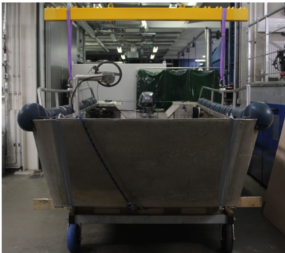
Figure 4 Inclining experiment rig
