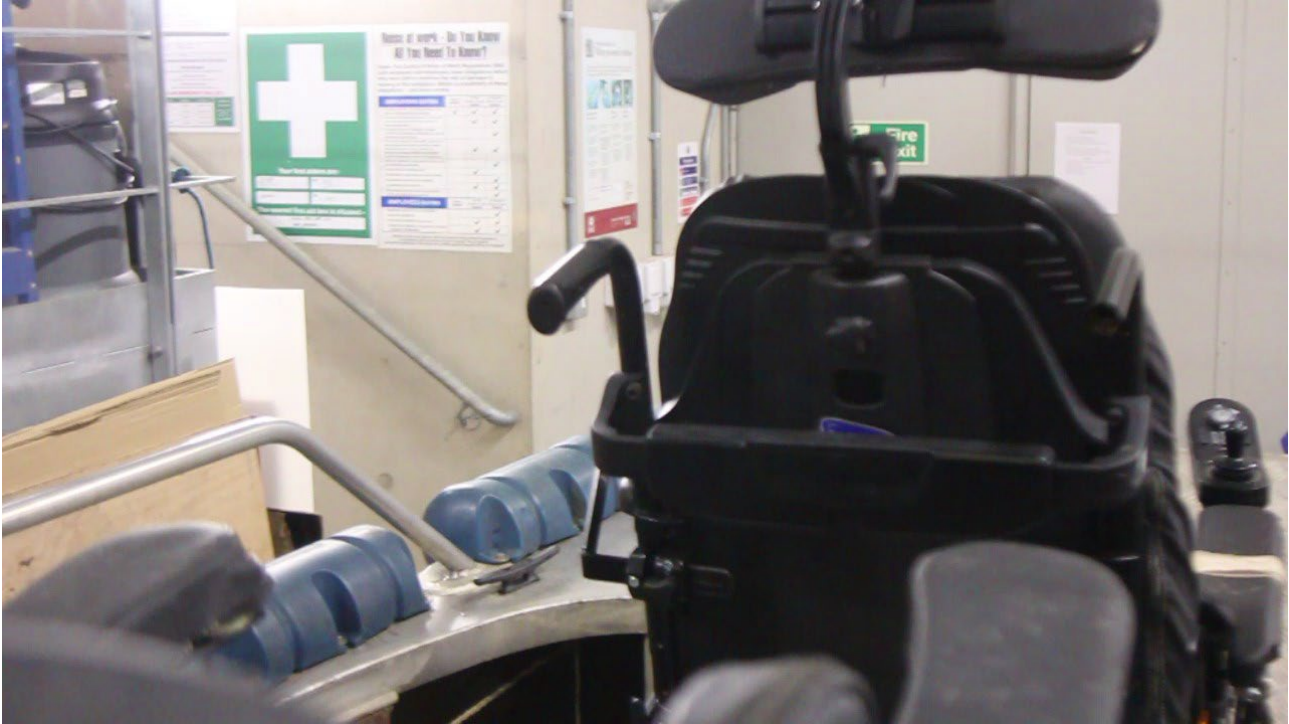
Figure 15 View of port side bow of Wheelyboat No.123 from central steering station, camera lens at eye level of a 1.63m tall person, seated behind helm, seat height 0.47m above the cockpit sole.
