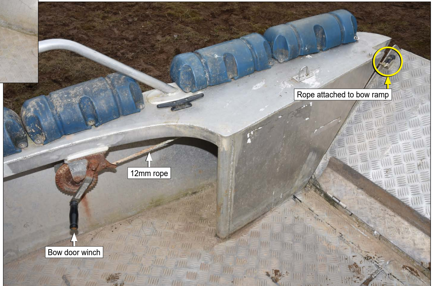
Figure 8: Bow door winch and safety clip
