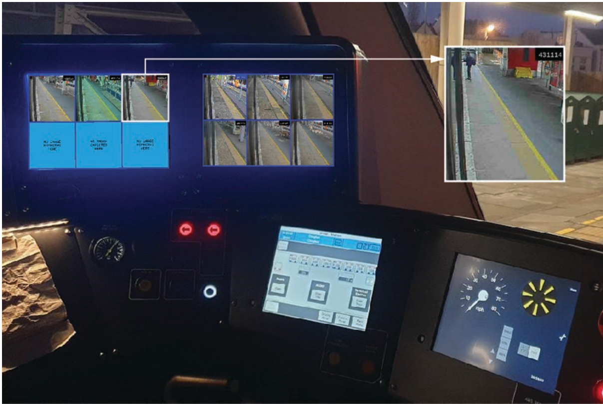
A class 710 driving cab with images from the monitors on the day of the accident superimposed by RAIB showing the passenger on the platform (courtesy of Arriva Rail London).
