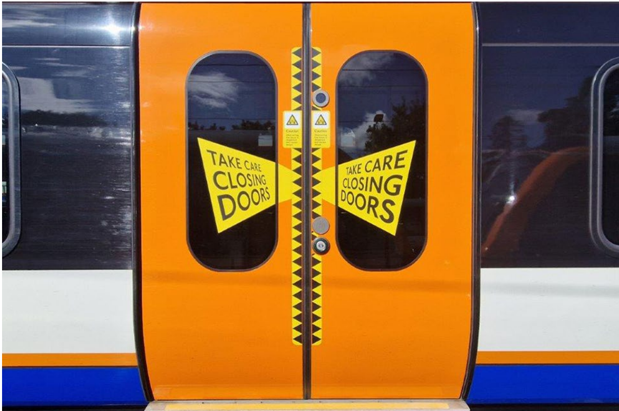
Doors on the side of a class 710 showing the ‘sharks teeth’ markings and warning labels (courtesy of Arriva Rail London).
