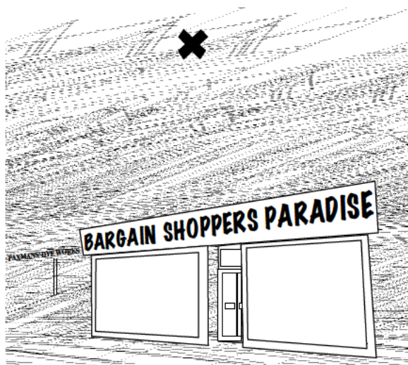
Overlarge fascia obscuring original fascia and spanning pilaster
