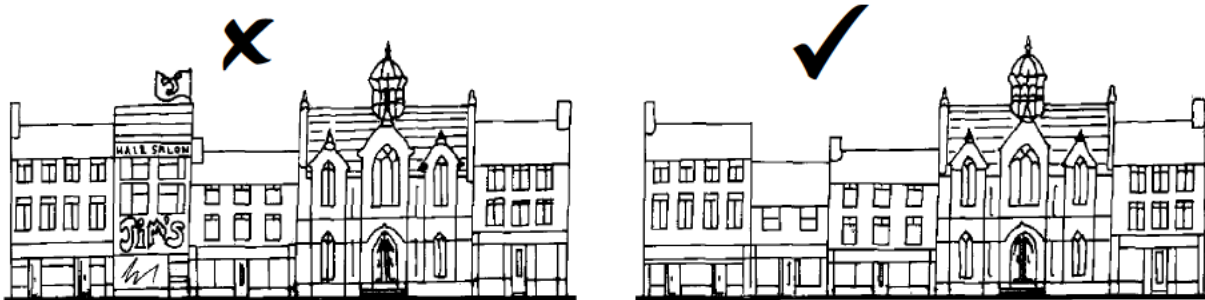
Jim's shop is too prominent in the street and detracts from the more important buildings
