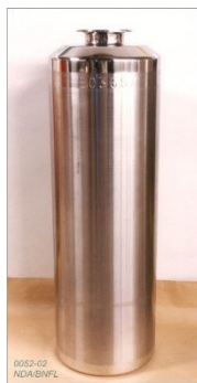
Figure 6: Example of HLW in a stainless steel WVP product container
