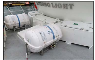
Guiding Light's survival equipment stored in boxes next to the liferafts
